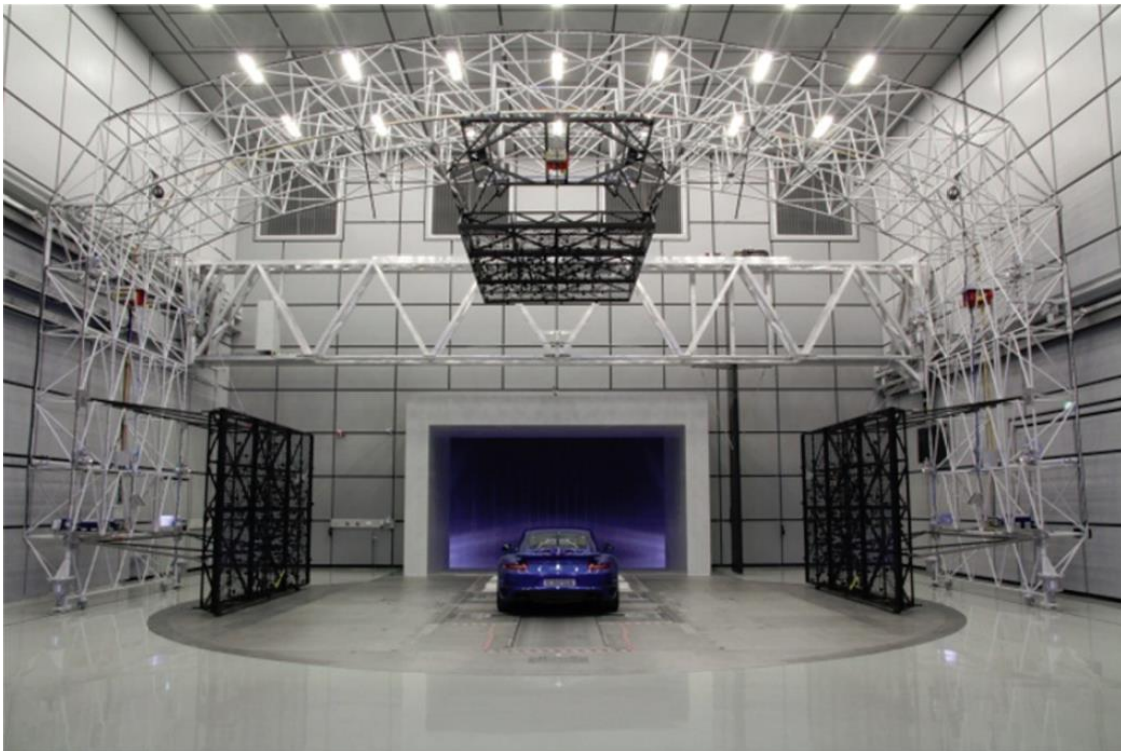
Fig. 3-7a: Example of a large microphone array consisting of three planar arrays in a wind tunnel [22]
