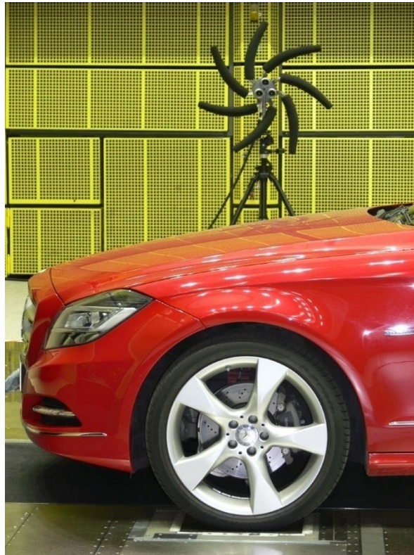
Fig. 3-7: Example for a mobile microphone array (source: FKFS)
