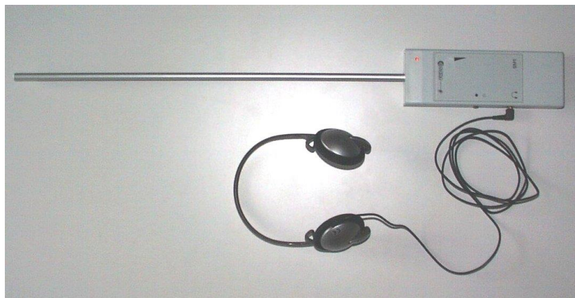
Fig. 3-9: Microphone probe with headphones
