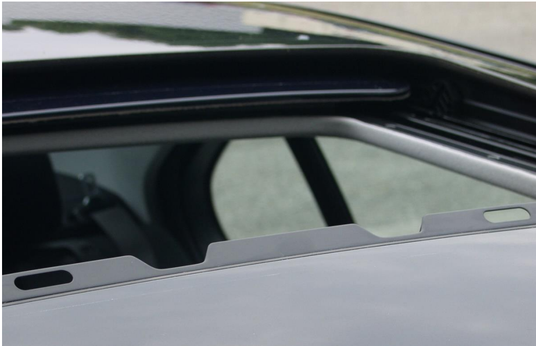
Fig. 4-11: Wind deflector with notches and apertures
