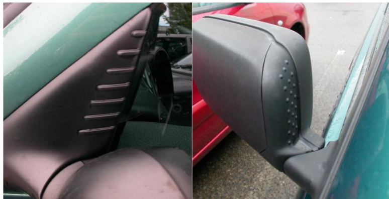
Fig. 4-2: Vortex generator to avoid tonal noise in the area of two exterior mirrors of production vehicles
