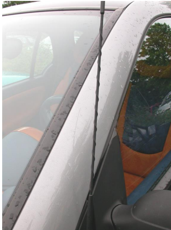
Fig. 4-6: Series antenna with wire spiral
