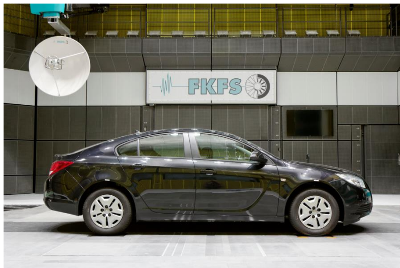
Fig. 3-8: Parabolic microphone in the measuring range of an aeroacoustic wind tunnel
