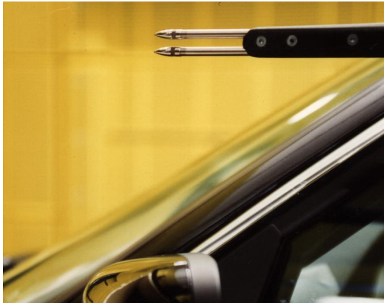
Fig. 3-5: Sound intensity probe with microphones with nose cones in parallel set-up above the exterior mirror of a passenger vehicle [8]
